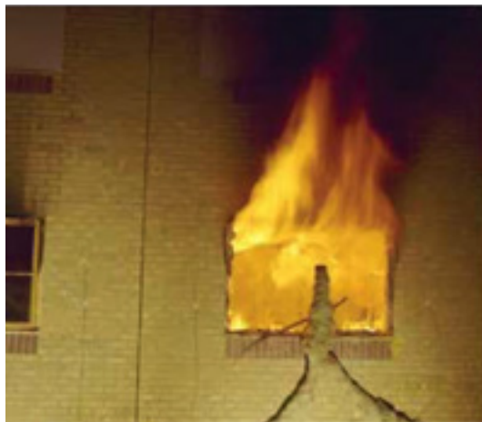
Figure 8. Fire coming through the opening on the building after flashover [10]
